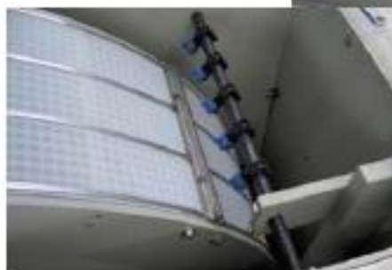
Samonac (33), automatic washing system, 150 PE
